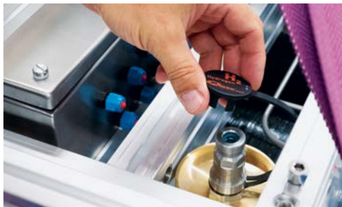
Measuring system for calibrating hydrogen filling stations.
