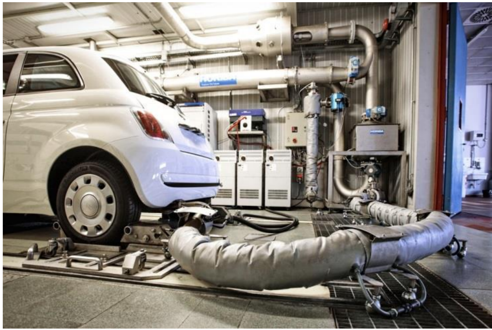
Fig. 1: Type approval of light vans and passenger cars according to Euro 5b and 6 relies on the measurement of particle number concentration. (Example image by airqualitynews.com)
